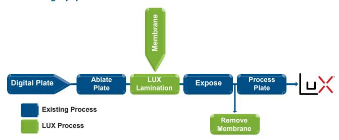
The LUX Laminator is a simple addition to your existing digital workflow. LUX Membrane 100 is laminated to the digital plate following laser ablation. This lamination process takes between 4-6 minutes, and works with all plates, including the largest available size, 52" x 80" (1321mm x 2032mm). Following exposure on your existing unit, the Membrane is peeled off and disposed in seconds. The plate can then be processed in your existing equipment.
